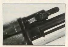
one turn in 9.6 inches. Total length of the barrel is 20.8 inches. Chambers and bores are chrome-plated. There is no muzzle device on the barrel and no grenade-launching capability. Somewhat heavy by today's standards, the weight, empty, is 8.6
